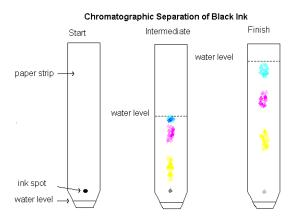
The black ink is made of three colours. each color has a different molecule size, then they will migrate at different velocities. Although the original colour of the ink was black, it is possible to see that this colour is made of three different colours. The same happens with the plants.
